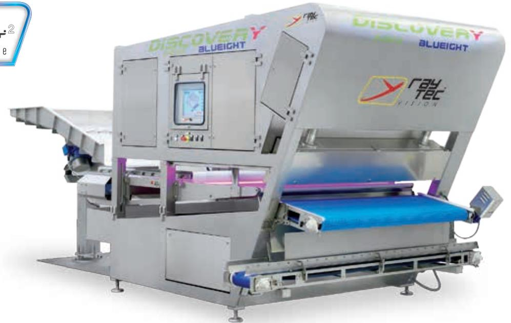
**SORTING MACHINES WITH CAMERA AND AIR-JET EXPULSION SYSTEM**
