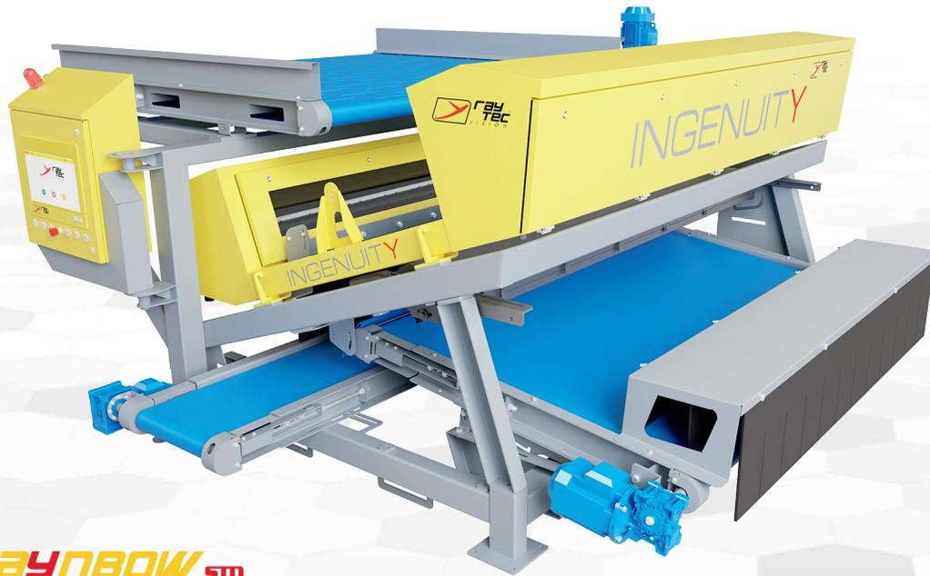
**INGENUITY** is a **double-vision sensor sorter**. It is equipped with Visible Color and NIR technology (Near Infra Red).
