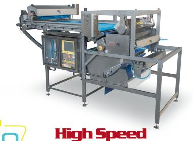
RAYNBOW is a high resolution sensor sorter. It is equipped with Visible Color and NIR technology (Near Infra Red). The system can detect the presence of organic or inorganic foreign bodies (including completely black), rotten products and color defects. Ethernet connection for remote access is available.
