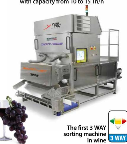
Top quality wine accept just sound and ripe grapes. The new multi-frequency sorter DIONYSOS automatically removes all contaminants from the inlet stream and ensure the top quality grapes to the wine process, up to a capacity from 10 to 15 Tn/h.
