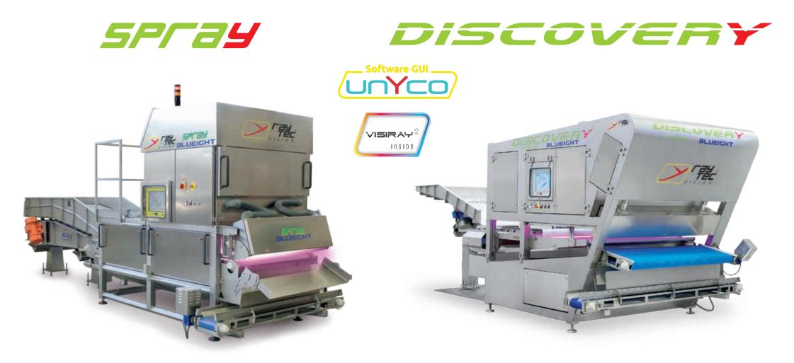
SORTING MACHINES WITH CAMERA AND AIR-JET EXPULSION SYSTEM Designed specially for controlling small-sized food products
